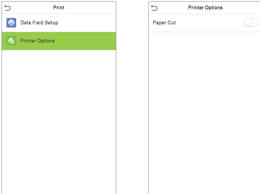
**Remarks:** To turn on the **Paper Cut** function, it is required to connect the device with a printer with paper cutting function, so that the printer will cut papers according to the selected printing information while printing.
