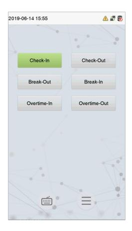
Press the corresponding punch state key to select your current punch state, which is displayed
